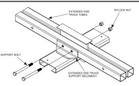
Diagram 5I. Assembling extended end truck.
