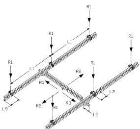
Diagram 1. Applied forces to supporting structure.
