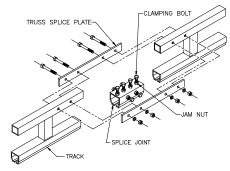
Diagram 4B. Splicing trussed track.
