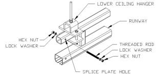
Diagram 3E. Hanger Retaining Bolt, 250#-2000#.
