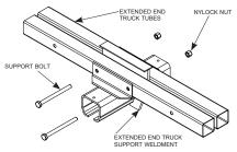
Diagram 5F. Assembling extended end truck.
