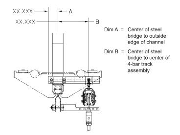
Diagram 10E. Steel bridge A-B dimensions.
