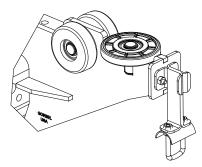
Diagram 5D. Installing tow arm on end truck.
