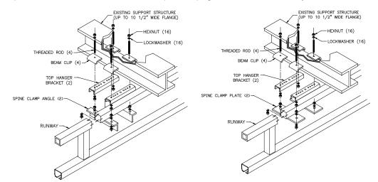
Trussed track with 3" to 6" top tube. Trussed track with 1-1/2" to 2-1/2" top tube. Diagram 2J. Installing Perpendicular Flush Mounted Hangers on trussed track.
