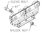
Diagram 6G. Installing hoist on loadbar hoist trolley.
