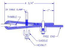
**Diagram 9D.** Saddling the cable on one end.
