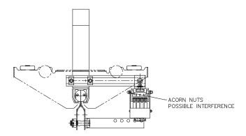
Diagram 10W. Universal electric possible endtruck interference.
