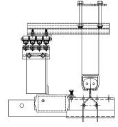
**Diagram 10T.** Conductix outside design for standard end trucks.
