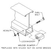
Diagram 5M. Installing end stop.
