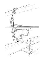
Diagram 11B. Safety cable installed on ceiling mounted hanger connection.
