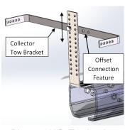
Diagram 10Q. Tow bracket directly mounted to mast.
