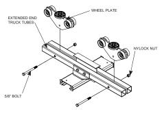
Diagram 5J. Installing wheel plates.
