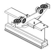
**Diagram 5B.** Installing clamping end truck on aluminum bridge. See **NOTE**.
