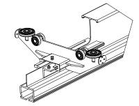
**Diagram 5C.** Installing clamping end truck on coped aluminum bridge. See **NOTE**.
