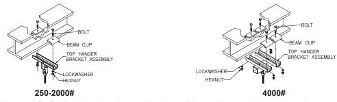
Diagram 2F. Bolting sloped top hanger bracket and beam clips to existing support beam.
