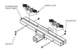
Diagram 5G. Installing wheel plates.
