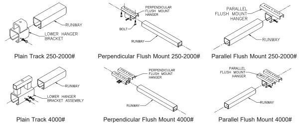
Diagram 2G. Installing lower hanger assemblies on untrussed (plain) track.
