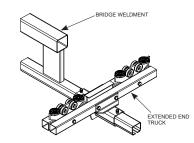
Diagram 5H. Installing extended clamping end truck. See NOTE.
