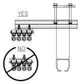
Diagram 10S. Conductix installation orientation.
