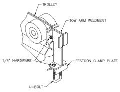
Diagram 6E. Installing tow arm on trolley.
