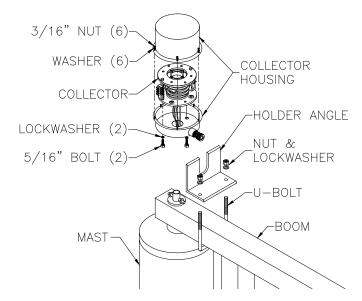
Diagram 9A. Installing electrical bottom entry collector.
