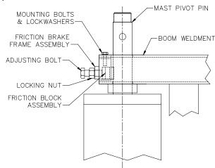
Diagram 8B. Installing friction brakes on WSJ360.
