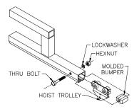
Diagram 5G. Installing hoist trolley and endstop.
