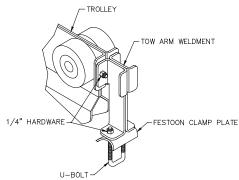
Diagram 5F. Installing tow arm on trolley.
