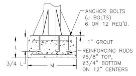
Diagram 3F. Hexagonal base plate foundation.
