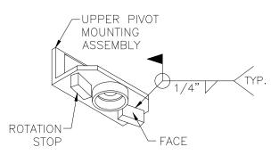
Diagram 9C. Welding rotation stops on the WSJ360.
