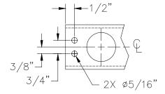
**Diagram 8C.** Retrofitting friction brakes on WSJ360.
