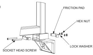
**Diagram 8A.** Installing friction brakes on Wall Mounted Work Station Jib.
