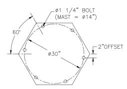
Diagram 3D. 6 bolt base bolt pattern.
