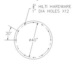
Diagram 3H. 44" dia. 12 bolt base bolt pattern.
