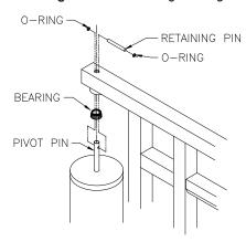
Diagram 4D. Installing boom weldment.
