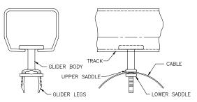
**Diagram 6A.** Installing electric cable on festoon glider.
