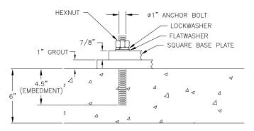
Diagram 3A. Typical square base plate anchor bolt embedment.
