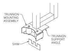
Diagram 4E. Adjusting trunnion rollers.
