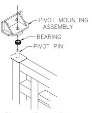
**Diagram 2D.** Installing upper pivot mounting assembly.
