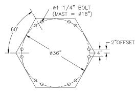
Diagram 3E. 12 bolt base bolt pattern.
