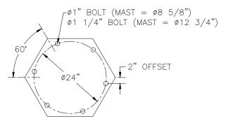
Diagram 3C. 6 bolt base bolt pattern.
