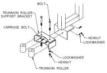
Diagram 4A. Installing trunnion rollers.
