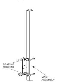
**3b.2** Slide boom assembly up along mast weldment for desired vertical position.
