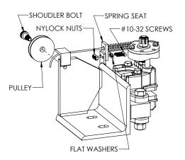
Diagram 7B. Attaching caliper to bracket. Diagram 7C. Assembling spring seat and pulley to bracket.
