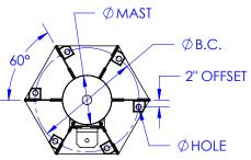
Diagram 3A. 6 bolt base bolt pattern.
