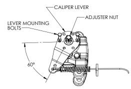
Diagram 7A. Brake caliper assembly.
