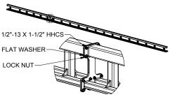
Diagram 5K. Plate style splice joint design.
