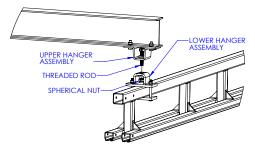
Diagram 5D. Attaching monorail to cantilever.
