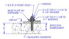
**Diagram 3D.** Anchor bolt installation.
