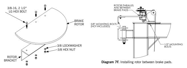
Diagram 7E. Attaching brake rotor to bracket.
