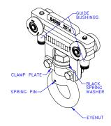
Diagram 6B. Recover trolley installation.
