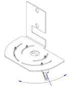
ADJUST LIMIT SWITCHES TO LIMIT SWING ARM COVERAGE
