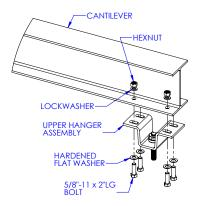
Diagram 5B. Attaching upper hanger to
