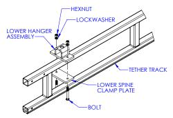
**Diagram 5C.** Attaching lower hanger assembly to monorail.
