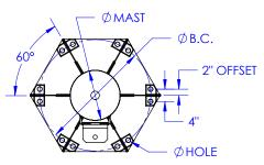
Diagram 3B. 12 bolt base bolt pattern.
