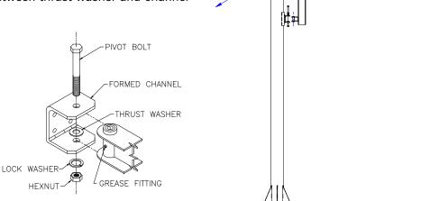
**Diagram 4A.** Attaching cantilever to mast.
