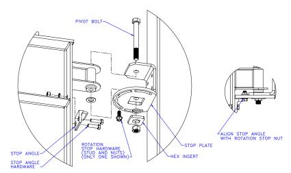
**Diagram 10A.** Rotation stop installation.
