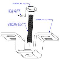
**Diagram 5A.** Assembling threaded rod to upper hanger.
