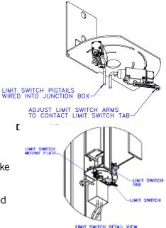
Diagram 9C. Limit switch detail.
