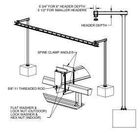
Diagram 5C. Installing under hung monorail.
