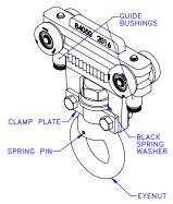
Diagram 6B. Recover trolley installation.
