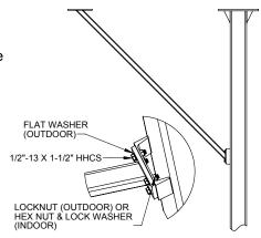
Diagram 3A. Installing knee brace.
