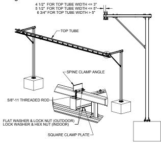
Diagram 5B. Installing threaded monorail.
