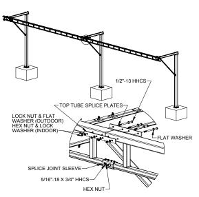
Diagram 5D. Sleeve style splice joint detail.
