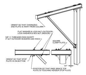
Diagram 4A. Orienting and installing header.
