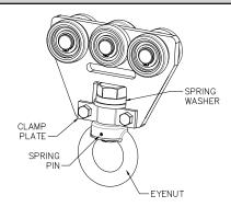
Diagram 6A. Tether Track® trolley installation.
