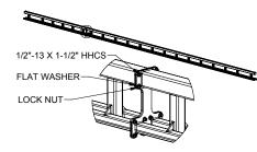
Diagram 5A. Plate style splice joint detail.
