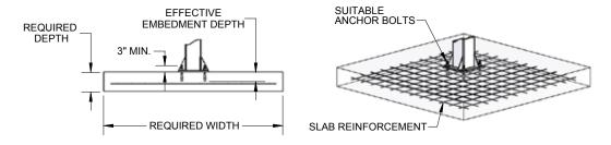
Diagram 2E. Post-installed shallow foundation detail.
