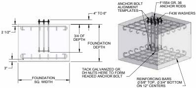
Diagram 2A. Cast-in Poured Foundation Detail.
