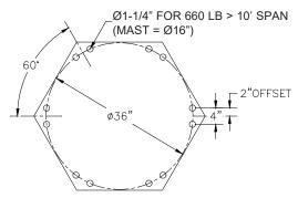
Diagram 3E. 12 bolt base bolt pattern.
