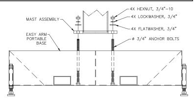
Diagram 10A. Column to portable base assembly.
