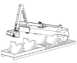
**Diagram 2D.** Easy Arm® assembly removal from packaging.
