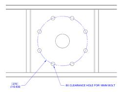
**Diagram 5B.** Bolt Pattern for Under Hung Easy Arm®.
