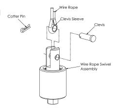
**Diagram N.** Removing wire rope from Pendant Handle.
