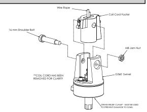
**Diagram 6B1.** *G*360<sup>™</sup>, *Shoulder Bolt and Coil Cord.*
