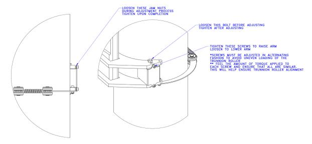
Diagram 4E. Trunnion roller adjustment.
