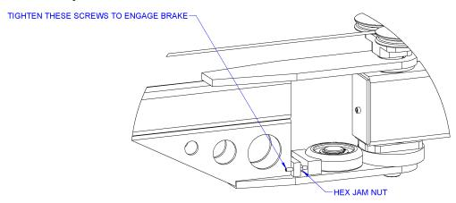
Diagram 8B. Secondary arm friction brake adjustment.
