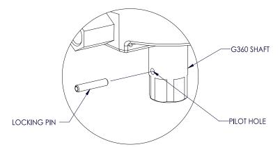
Diagram 6B2. Tooling Installation.
