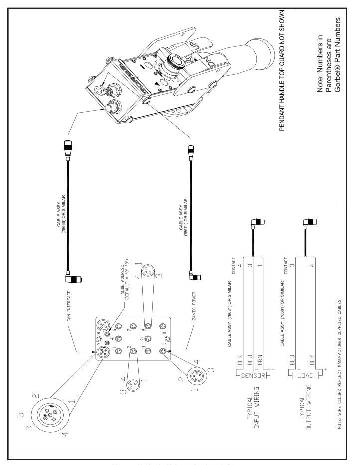
Diagram K. Handle IO Detail, Pendant Model.
