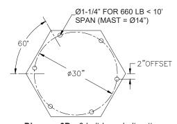
Diagram 3D. 6 bolt base bolt pattern.
