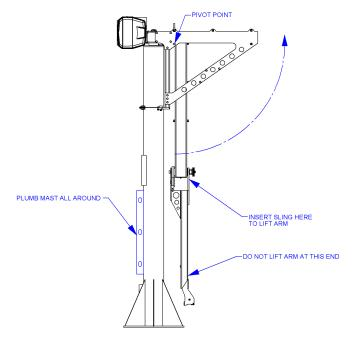
Diagram 4A. Final arm assembly installation.
