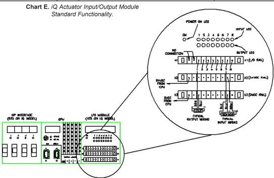
Diagram F. Actuator CPU Input/Output Block.
