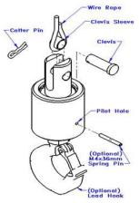
**Diagram 6C3.** Cotter Pin, Clevis, Wire Rope Swivel Assembly and Wire Rope Thimble.
