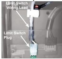
Diagram P. Gently pull out the grey limit switch wiring lead to disconnect plug from board.
