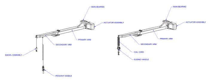
Diagram 1B. Main Under Hung Easy Arm® Components.
