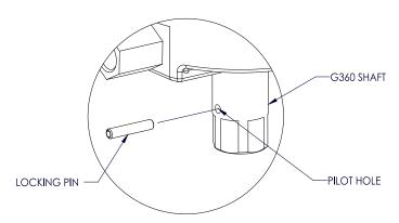
Diagram 6D2. Tooling Installation.
