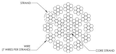
Diagram L. 19x7 Preformed Wire Rope Composition.
