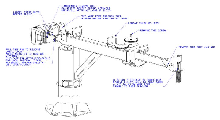
Diagram W. 660# Easy Arm wire rope replacement.
