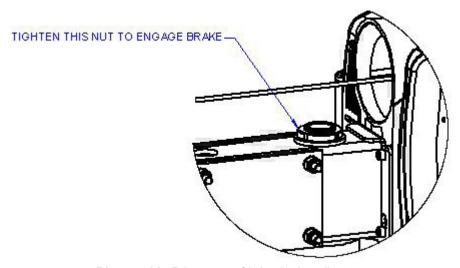
Diagram 8A. Primary arm friction brake adjustment.
