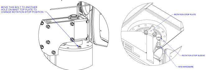
Diagram 8C. Floor mounted arm assembly rotation stop installation.
