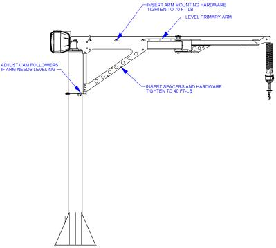
Diagram 4B. Arm assembly-leveling adjustment.
