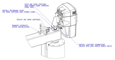
Diagram 4D. Installing electrical connector.
