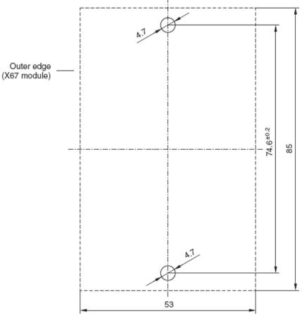
Diagram 13B. Screw fastener drilling template.
