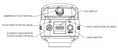
Diagram B. Slide Handle - G-Force® Logo (Float Mode), MENU and Emergency-Stop Buttons and LEDs.
