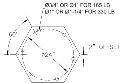
Diagram 3C. 6 bolt base bolt pattern.
