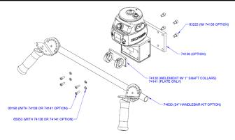
Diagram 6F1. Mounting handlebar and mounting plate.
