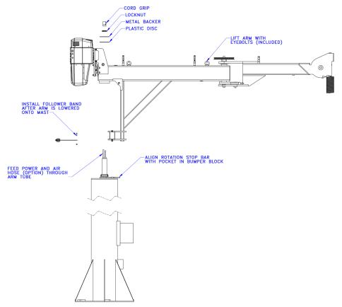
Diagram 4C. Aligning arm with mast.
