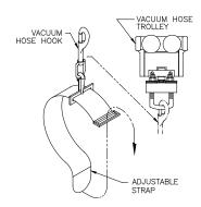
**Diagram 8F.** Installing vacuum hose on vacuum hose trolley.
