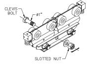
Diagram 61. Installing hoist on A150 hoist trolley.
