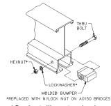
Diagram 4C. Installing standard endstop.
