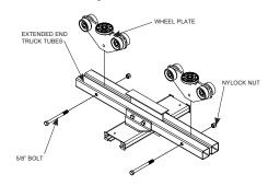
Diagram 5F. Installing wheel plates.
