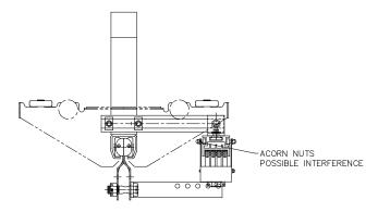
Diagram 10S. Universal electric possible endtruck interference.
