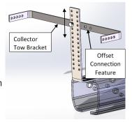
Diagram 10L. Tow bracket directly mounted to mast.
