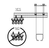
**Diagram 10N.** Conductix installation orientation.
