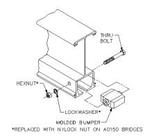
Diagram 5H. Installing end stop.
