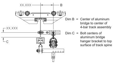
Diagram 10E. One piece aluminum bridge B-C dimensions.
