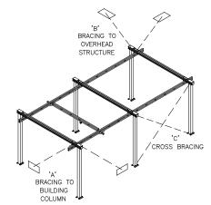
**Diagram 1.** Examples of typical sway bracing locations.
