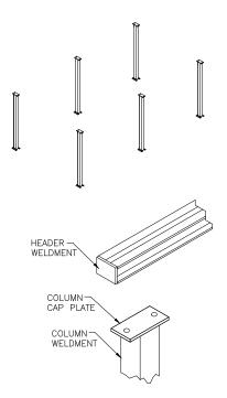
**Diagram 2A.** Orienting column cap plate.
