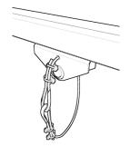
**Diagram 11C.** Safety cable installed on Gorbel® trolley that will attach to hoist (by others).
