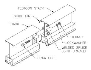
Diagram 7A. Installing festoon stack section.
