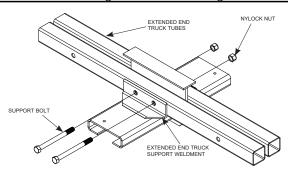
Diagram 5E. Assembling extended end truck.
