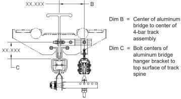
Diagram 10F. Two piece aluminum bridge B-C dimensions.
