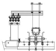
Diagram 10Q. Conductix inside design for extended end trucks.
