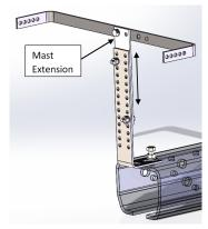
**Diagram 10M.** Mast extension configuration.
