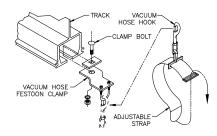
**Diagram 8C.** Installing vacuum hose clamp on runway or bridge.
