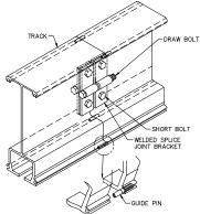
Diagram 4B. Splicing Aluminum track sections.
