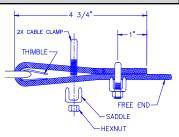
Diagram 11A. Saddling the cable on one end.
