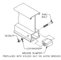
**Diagram 7B.** Re-installing endstop in track after installing festoon stack section.
