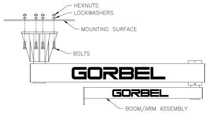
Diagram 2A. Crane Installation.
