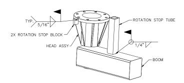
Diagram 3B. Welding Boom rotation stop.
