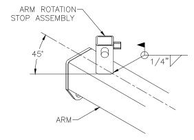
Diagram 3A. Welding arm rotation stop assembly.
