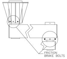
Diagram 2B. Friction brake bolt location.
