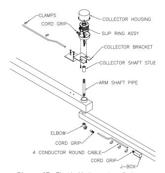
Diagram 3E. Electrical bottom entry collector.
