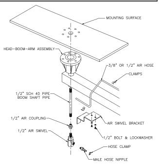
Diagram 3D. Boom Air Swivel Assembly.
