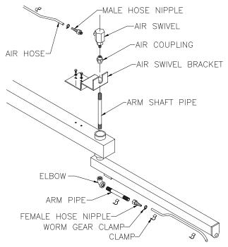
Diagram 3F. Bottom entry air-swivel assembly.
