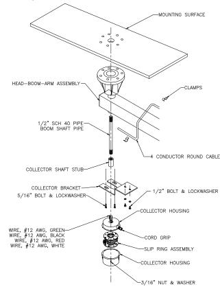
Diagram 3C. Boom Electrical Bottom Entry Collector.
