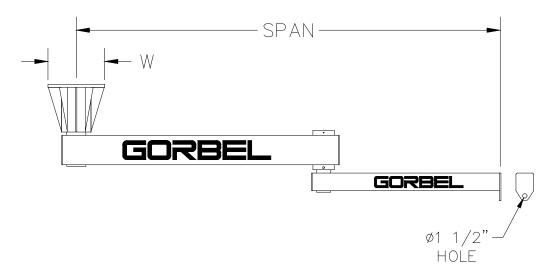
Diagram 1A. Ceiling Mounted Articulating Jib Crane.
