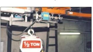
This monorail system shows a Tri-Bar entrance guide and a Power Pickup on a disengageable base. The hoist is entering an electrified zone for a hoisting area.
