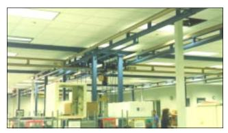
Eliminate low hanging, unsightly festoon cords and tag lines, with compact Tri-Bar on this light duty crane, at this electronics manufacturer.
