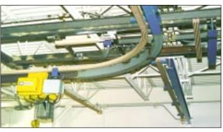
Four-Bar is perfectly formed to any curve, switch and transfer requirement. Systems are custom fabricated to customer requirements.
