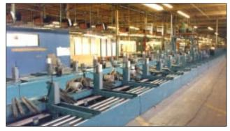
Another appliance manufacturer has 166 moving carriers for evacuation and burn-in testing on a loop. Another brand of conductor rail was replaced after giving trouble ever since it was installed. Four-Bar has operated with total satisfaction.
