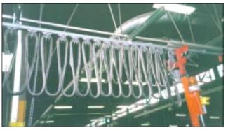
A corrugated products manufacturer had trouble with festoon systems failing on their transfer cars due to air contaminants and frozen trolleys.
