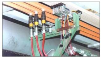
10 control lines require less than 7 inches of space for this steel slab grinder, using Tri-Bar and Four-Bar. Universal's Span-Guard, shown, provide the main power.
