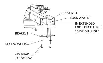
Diagram 3B. Extended End Truck Mounting Bracket.
