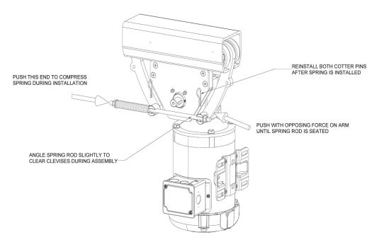
Diagram 4A. Installation of Tractor Drive.
