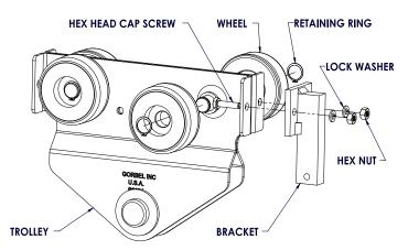
Diagram 3A. Hoist Trolley/End Truck Bracket Mounting.
