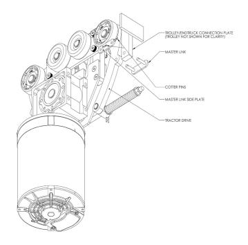
Diagram 6A. Link Pin Installation.
