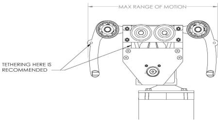
Diagram 4B. Installation of Tractor Drive.
