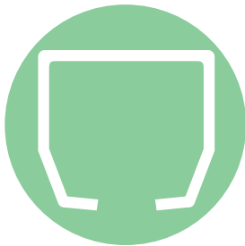
2-degree taper keeps the trolley centered
